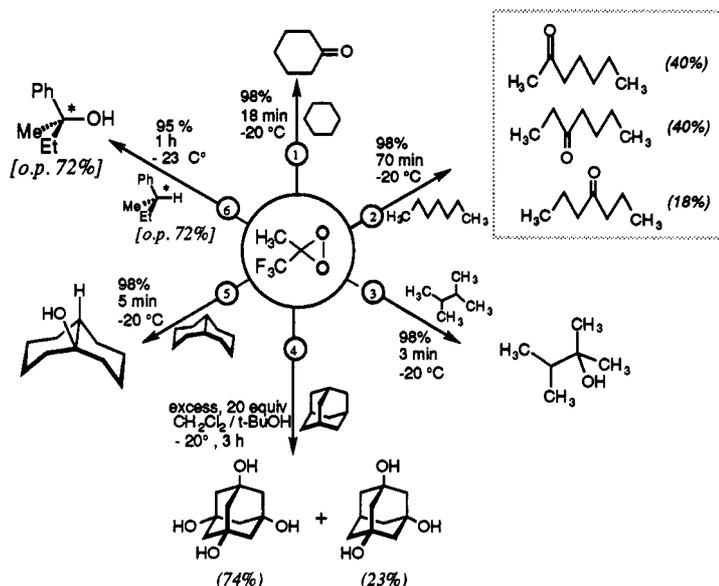
Fig. 3 Efficient oxyfunctionalization of alkanes using methyl(trifluoromethyl)dioxirane (**1b**)
