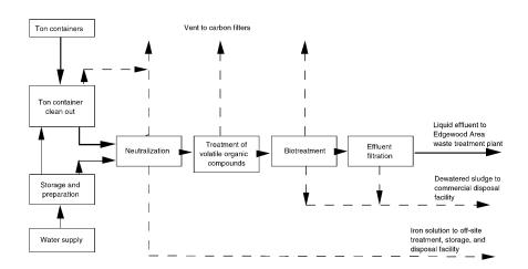
Fig. 3 Configuration for mustard hydrolysis and on-site biotreatment for Aberdeen Chemical Disposal Facility.
