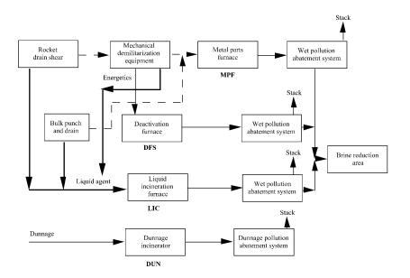
Fig. 1 U.S. baseline incineration system<sup>a</sup>.
