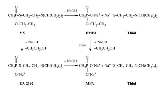
Fig. 5 Reaction scheme for neutralization of VX with sodium hydroxide.
