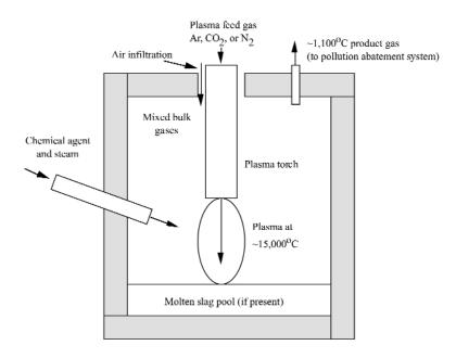
Fig. 2 Typical plasma waste converter.
