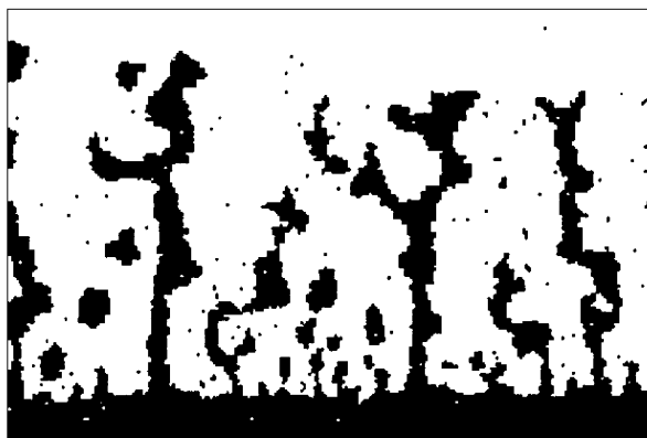
Fig. 9 Monte Carlo simulation of the interface between two ion conductors in an electric field (black: good ionic conductor, white: bad ionic conductor, bottom: anode, top: cathode) [38].
