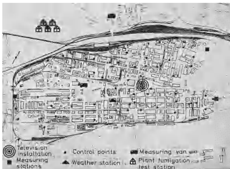
Figure 7. Air pollution surveying and control system in a chemical plant (by courtesy of the Farbwerke Hoechst AG)
