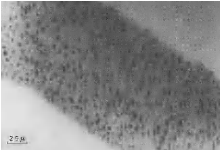
Figure 7. Section of an extracted membrane (PAA = 12 per cent) (transmission).
