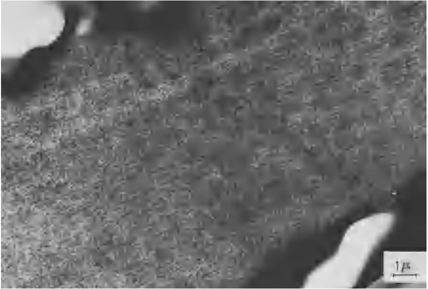
Figure 6. Section of an extracted membrane (PAA = 57 per cent) (transmission).
