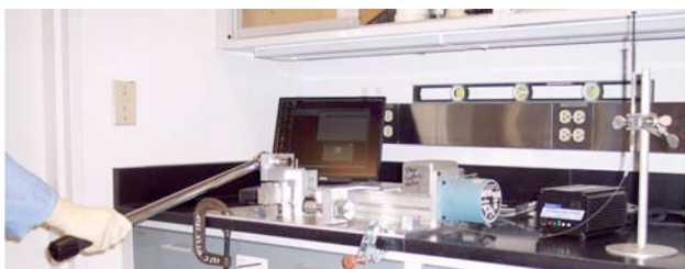
Semi-automated squeeze and cut system
