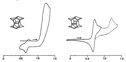
Fig. 6. CV's of 1 and 2 (standard conditions: CH<sub>2</sub>Cl<sub>2</sub>, 0.1 M TBAF<sub>6</sub>,  $\underline{v} = 100$  mV/s, vs. Ag/AgCl, r.t.).
