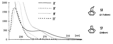
Fig. 3. UV absorption curves of 2', 5', 6' and 11' (CH<sub>3</sub>CN).
