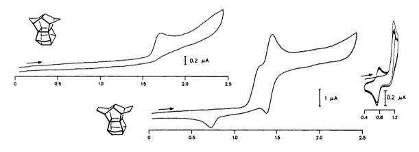
Fig. 7. CV's of iso-1 and iso-3 (CH<sub>2</sub>Cl<sub>2</sub>, 0.1 M TBAF<sub>6</sub>,  $\underline{v}$  = 100 mV/s, vs. Ag/AgCl, -30°C).
