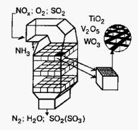
Fig. 6. Reactor and honeycomb catalyst for the catalytic reduction of  $NO_x$  in flue gases of power plants.
