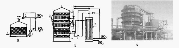
Fig. 7. Schemes and relative sizes of catalytic reactor and heat exchanger units for unsteady-state (a) and traditional steady-state (b) performance of  $SO_2$  removal from flue gases of non-ferrous metal plants (1 - reactor, 2 and 2' - three way values; 3 - catalyst beds; 4 and 5 - heat exchangers). Photograph of the industrial unit for unsteady-state  $SO_2$  removal (c).
