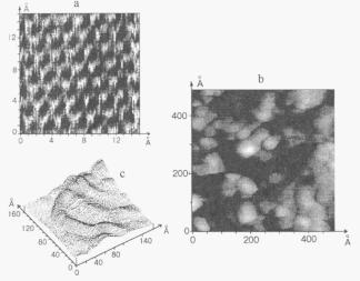
Fig. 1. STM images of: (a) - the basal surface of graphite; (b) - the surface of Pd/Sibunite catalyst with highly dispersed Pd particles; (c) - the surface of a large Pd particle in Pd/Sibunite catalyst.
