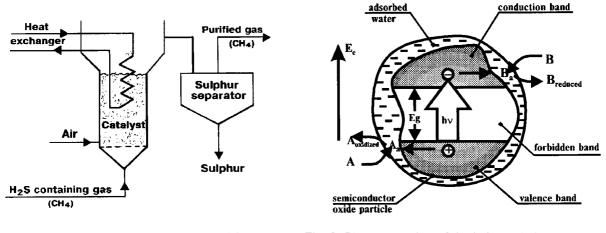
Fig. 8. Reactor with fluidized catalyst bed for selective oxidation of hydrogen sulfide.
