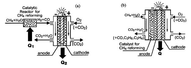
Fig. 4. High output methane fuel cells with the external (a) and internal (b) reforming of  $CH_4$ . Thick arrows indicate heat fluxes. M is the high-temperature oxygen conducting membrane or molten carbonate.
