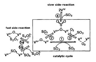
Scheme 2. The mechanism of  $SO_2$  oxidation to  $SO_3$  over industrial vanadium catalysts.
