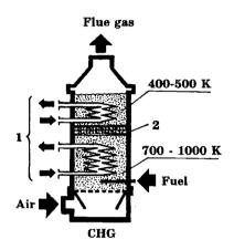
**Fig. 3.** A Catalytic Heat Generator (CHG) for heating/evaporation of liquids: 1 - heated liquid; 2 - temperature regulating grid.
