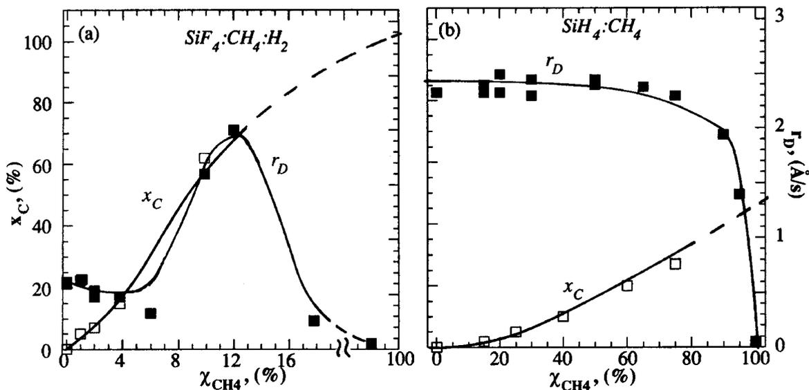
Fig. 2(a-b). Carbon content  $x_C$  ( $\text{C}/(\text{C}+\text{Si})$ ) and deposition rate  $r_D$  vs gas compositional ratio,  $\chi_{\text{CH}_4}$  ( $\text{CH}_4/(\text{CH}_4+\text{SiX}_4)$ ), for (a)  $\text{SiF}_4:\text{CH}_4:\text{H}_2$  and (b)  $\text{SiH}_4:\text{CH}_4$  (from ref. 23) mixtures.
