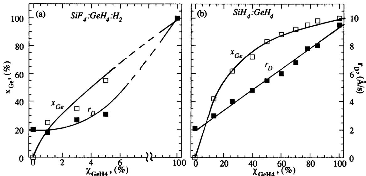
Fig. 1(a-b). Germanium content  $x_{Ge}$  (Ge/(Ge+Si)) and deposition rate  $r_D$  vs gas compositional ratio,  $\chi_{GeH_4}$  (GeH<sub>4</sub>/(GeH<sub>4</sub>+SiX<sub>4</sub>)), for (a) SiF<sub>4</sub>:GeH<sub>4</sub>:H<sub>2</sub> and (b) SiH<sub>4</sub>:GeH<sub>4</sub> (from ref. 21) mixtures.
