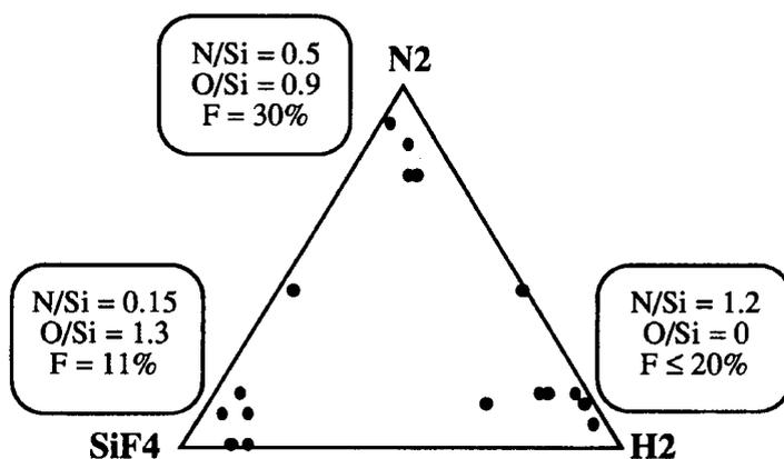
Fig. 4.  $\text{SiF}_4:\text{N}_2:\text{H}_2$  ternary diagram showing the various gas feed mixtures used for the deposition experiments. Chemical composition data refer to typical films deposited from  $\text{SiF}_4$ ,  $\text{N}_2$  and  $\text{H}_2$  rich mixtures ( $p = 1\text{ Torr}$ ,  $W = 50\text{ watt}$ ,  $T_D = 300\text{ }^{\circ}\text{C}$ ).
