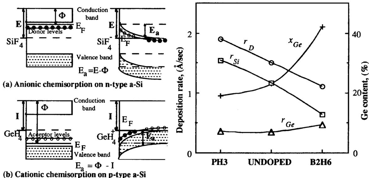
Fig. 3. Energy band structure and band bending at the surfaces of a n- and p-doped a-SiGe:H,F film in the case of  $\text{SiF}_4$  anionic chemisorption (a) and  $\text{GeH}_4$  cationic chemisorption (b), respectively. Total deposition rate ( $r_D$ ), Si and Ge partial deposition rate ( $r_{\text{Si}}$ ,  $r_{\text{Ge}}$ ), and Ge content ( $x_{\text{Ge}}$ ) for undoped and doped a-SiGe:H,F films from  $\text{SiF}_4$ - $\text{GeH}_4$ - $\text{H}_2$  plasmas.
