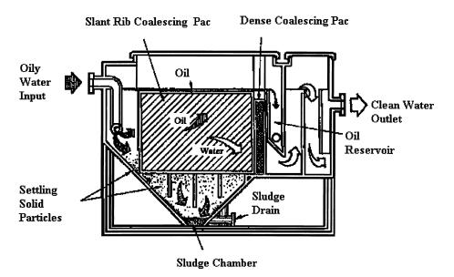
Fig. 2 Slant rib coalescing separator.
